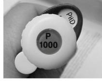
The limits are: P10: 1.0 - 10.0 µl P20: 2.0 - 20.0 µl P200: 20 - 200 µl P1000: 200 - 1000 µl
